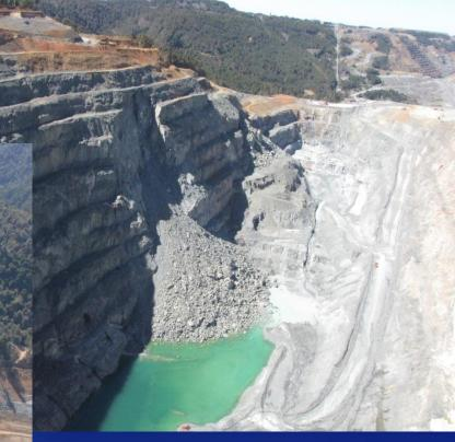
As a result of the wall failure, access to the high grade North Pit was cut off
