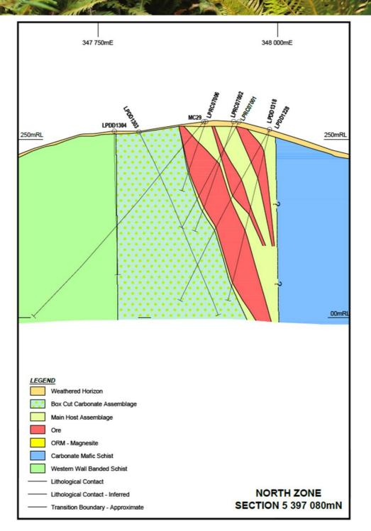
Figure 11 Long Plains Typical Cross Section
