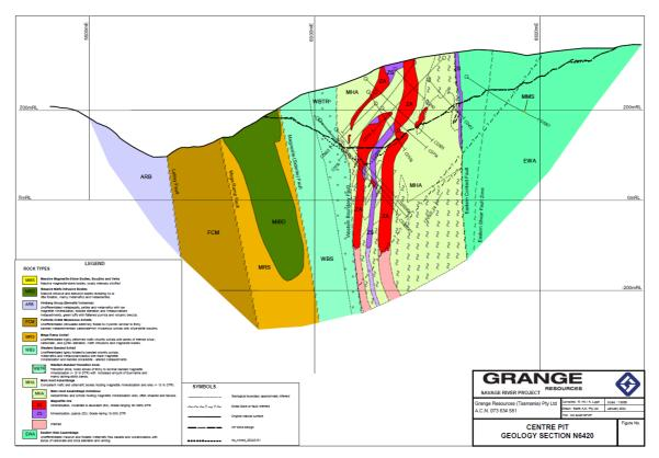
**Figure 9 Centre Pit Typical Cross Section**
