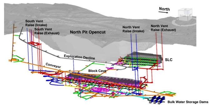
Figure 5 DFS design for the North Pit Underground Mine
