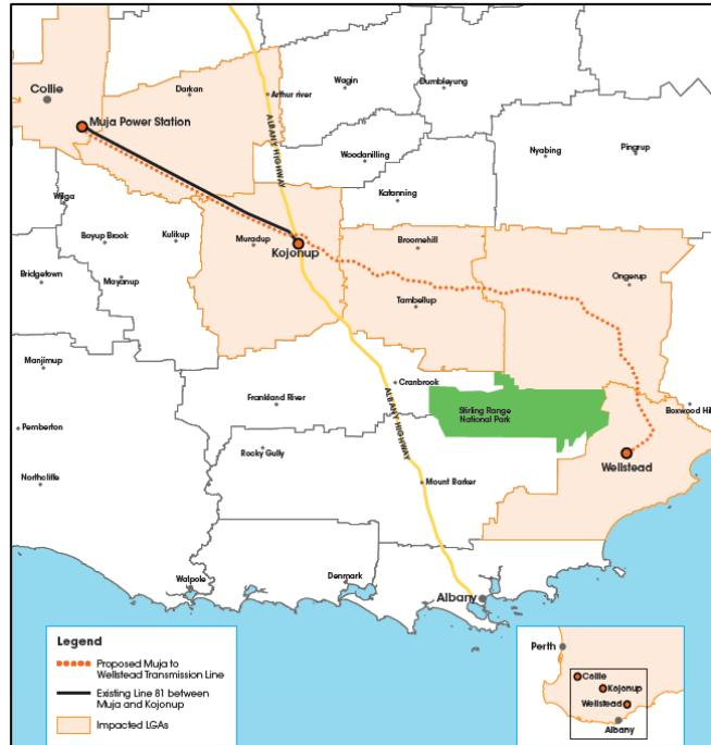
*Figure 5: Proposed Transmission Line Route for the 5mtpa PFS 2022*
