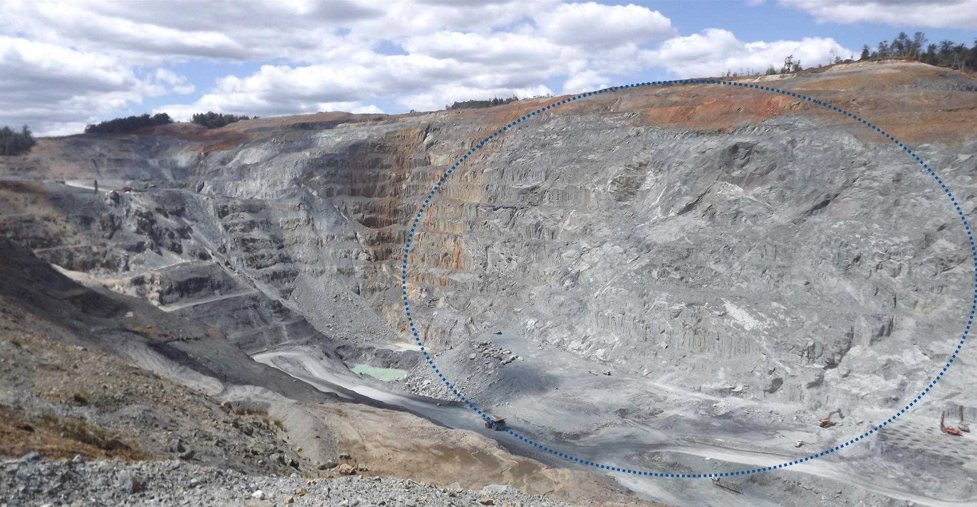
The East Wall has undergone a cut back and access to the North Pit has been re-established
