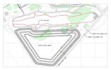
Figure 2: Layout of open pit and waste dump
